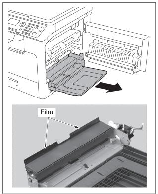
(5) Remove the indicated cover from the cover removed in step (4). (One screw)
