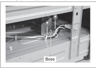
(24) Connect the connector of the cooling fan assembly to the main body.
