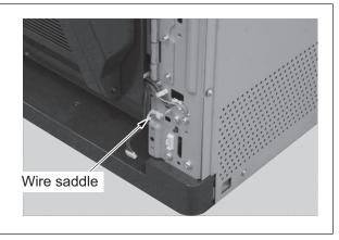
(17) Plug in the connector of the automatic duplex unit and route its cable through the wire saddle.
