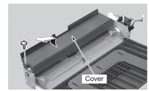
(6) Attach the supplied transport guide. (One supplied screw A)
