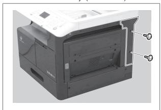
(3) Remove the indicated cover from the right door of the main body. (Two screws)
