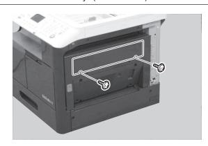
(4) Perform the following procedure.<When the multi bypass tray is not installed>a) Remove the indicated cover from the lower right side of the main body. (Two screws)
